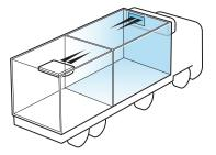
Multiline 8MT is 1100 mm wide and can be mounted in several places. A suitable solution for a movable partition that divides the box crosswise.
