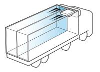
Multiline 7MTL is a slim unit - only 800 mm wide (one pallet width). It can be fitted in a refrigeration corridor both at the front and the rear.
