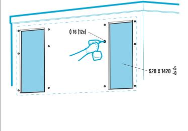
! The surface behind the machine should be free of strips, etc. If there are any strips, the machine must be shimmed to an even level. **INSTALLING ON THE BODY**
