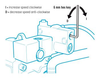
NOTE: The locking screw must be removed before making any adjustments. See point 23.
