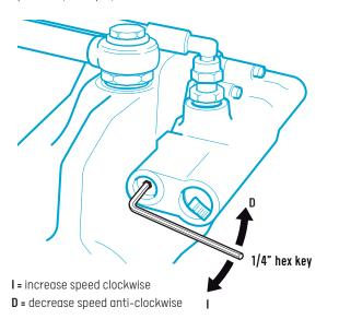
NOTE: The plug may only be loosened and installed when the vehicle engine is switched off.
