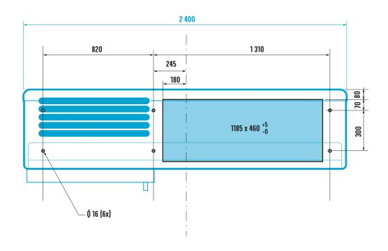
HH16 DRILLING DIMENSIONS headboard. All dimensions are in mm.
