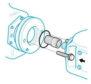
NOTE: The spline socket must be lubricated with engine oil before installation.
