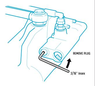
NOTE: The plug may only be loosened and installed when the vehicle engine is switched off.
