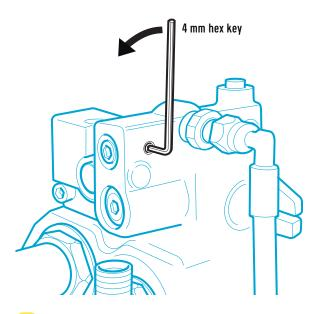
! NOTE: The locking screw must be removed before making any adjustments.
