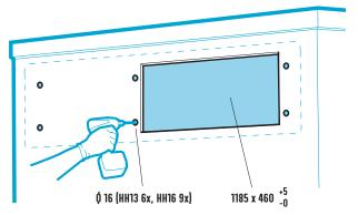
! The surface behind the machine should be free of strips, etc. If there are any strips, the machine must be shimmed to an even level.
