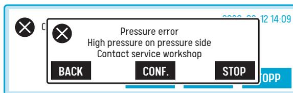
When the pressure error has disappeared and been acknowledged, the text **"No indicated errors"** is displayed.
