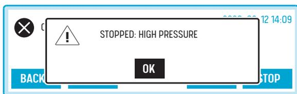
When a error message is displayed, press the **OK** button (the middle button) to confirm that you have seen the message.
